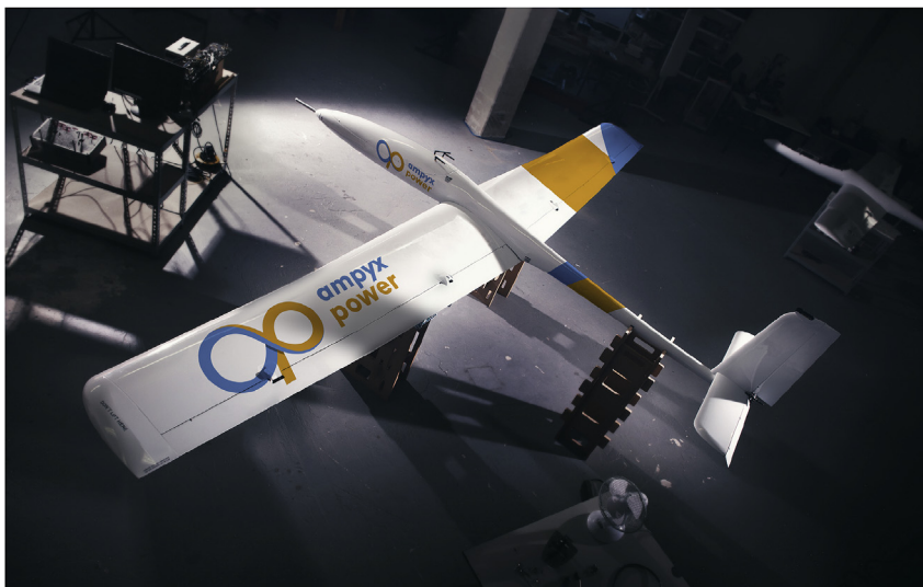
Fig. 2. The 2 nd prototype high lift, rigid wing autonomous aircraft designed by Ampyx Power B.V [5], and build in 2009.
