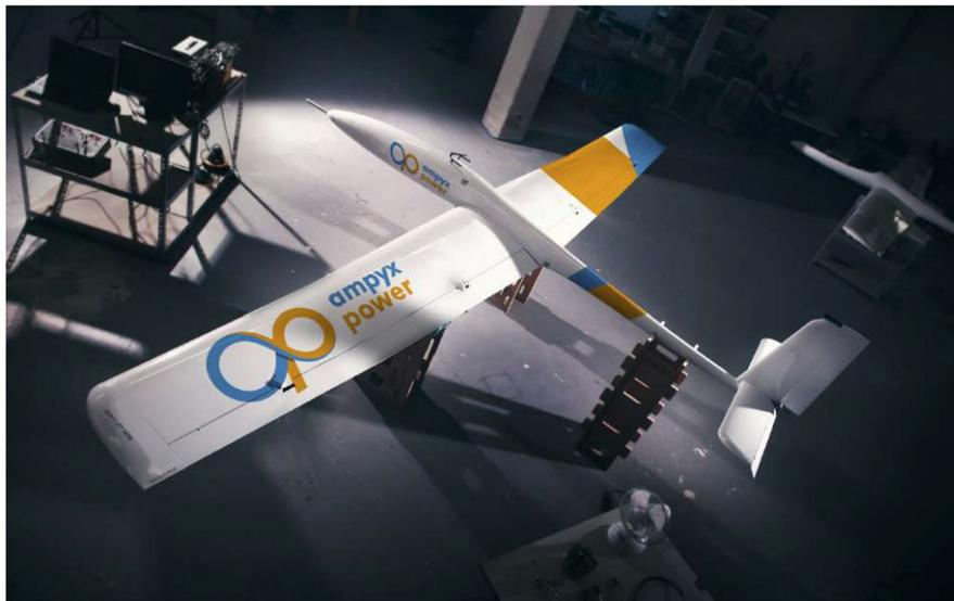
**FIGURE 1** The second prototype high lift, rigid-wing autonomous aircraft designed by Ampyx Power B.V. [Colour figure can be viewed at [wileyonlinelibrary.com](http://wileyonlinelibrary.com)]
