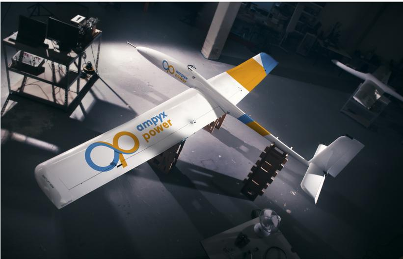
Figure 1.3: The 2<sup>nd</sup> prototype high lift, rigid wing autonomous aircraft designed by Ampyx Power B.V. [3].
