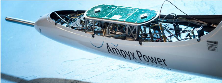
Figure 3.3: Five hole pitot tube and FCC mounted at the nose and inside the fuselage, respectively.
