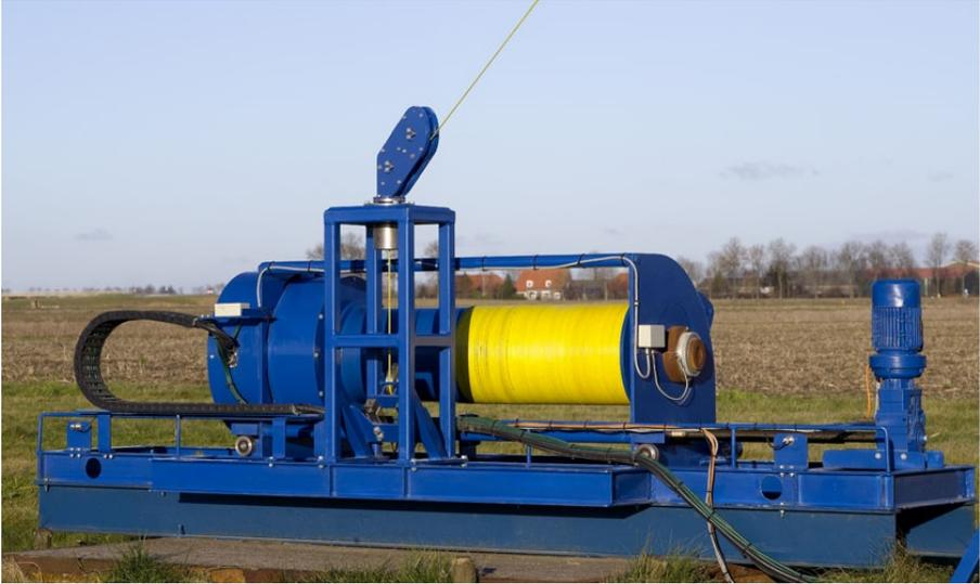
Figure 2.7: The ground station converts the mechanical energy from tether tension into electrical power and feeds it to the grid.
