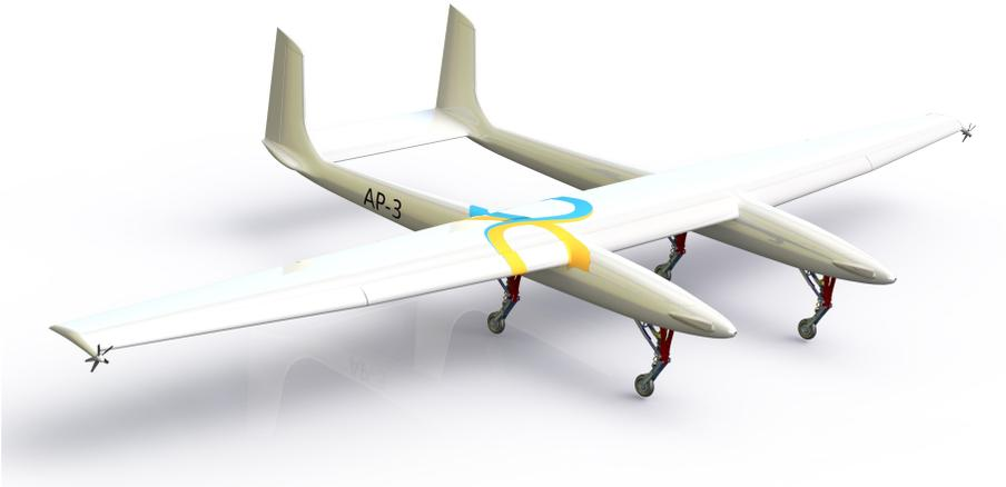
Figure 1.4: The 3<sup>rd</sup> prototype high lift, rigid wing autonomous aircraft designed by Ampyx Power B.V [3] (side view).
