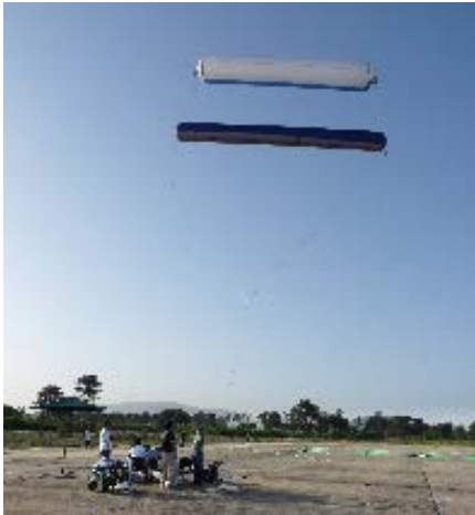
(c) AWE system using the Magnus effect [77].
