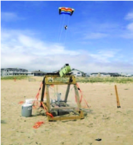
(d) Kite-Powered Water Pump during field testing [74].
