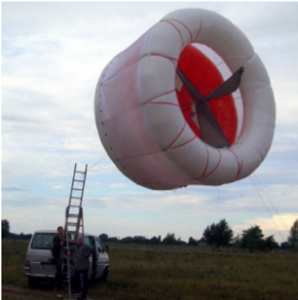
(b) System relying solely on aerostatic lift [93].
