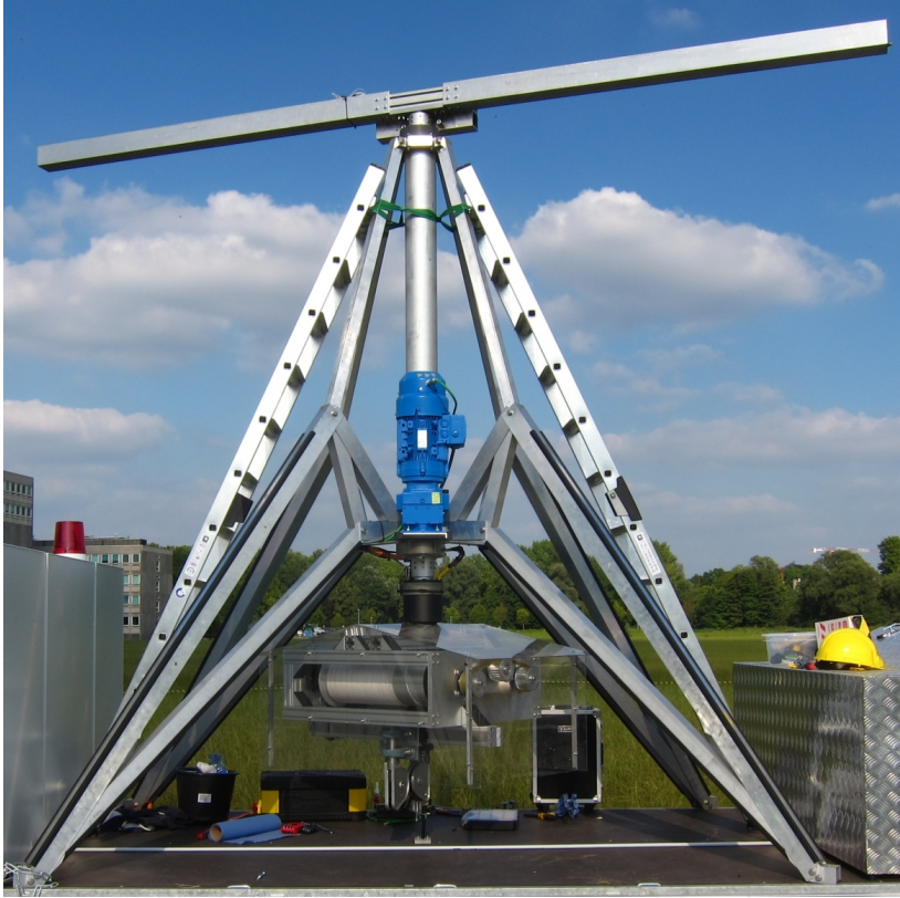
Figure 3.8: The designed and built outdoors carousel.
