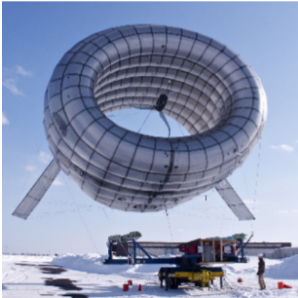
(a) System with wing-shaped duct [93].
