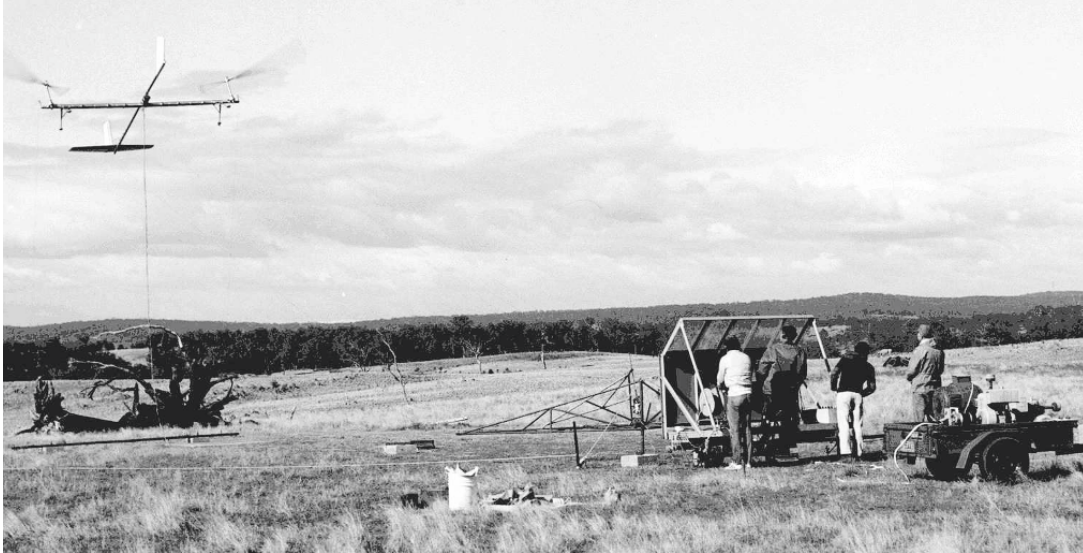
Fig. 1.2 Prototype testing the flying electric generators in Australia in May 1986, showing the powered craft almost in autorotation at a wind speed of 8 m/s. Electricity generation was achieved briefly in another test. The craft, which had a total mass of 29 kg, had two rotating hubs, each radiating a lifting rotor blade and a shorter streamlined blade with a counter-balancing mass at its tip (Photo by Bryan Roberts, provided by PJ Shepard).
